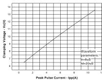
Clamping Voltage vs. Peak Pulse Current
