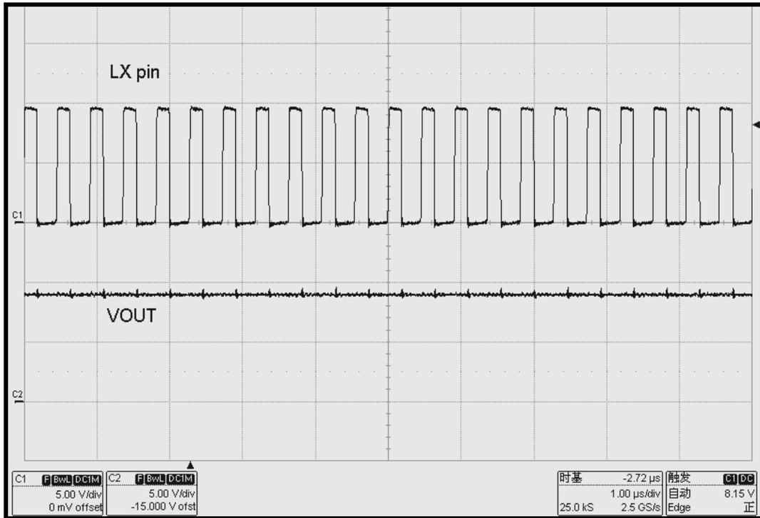
Fig 2.1 Output waveform diagram ( $V_{in}=3.6V$ , 3 pcs LED load)
