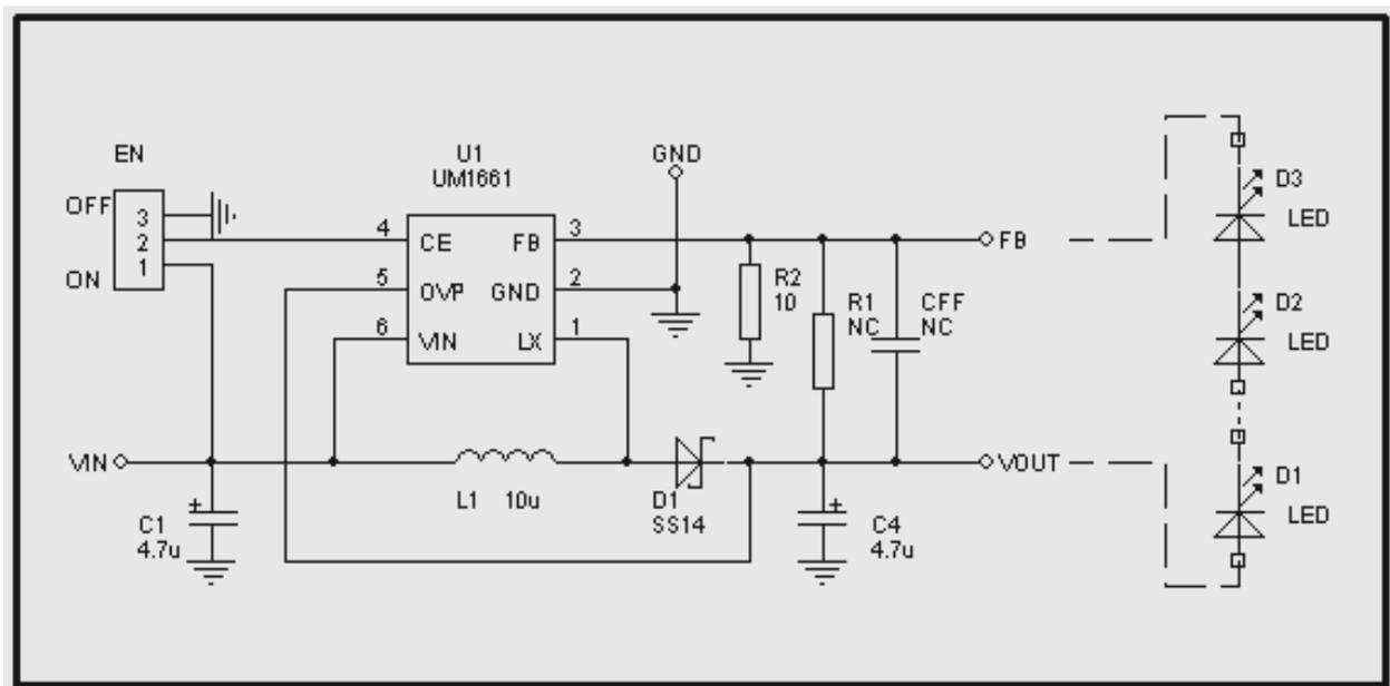
Fig 1.1 UM1661 EVB board schematic
