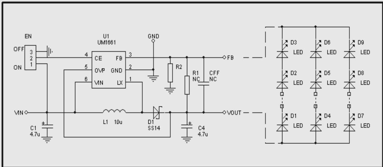
**Fig 5.1 UM1661 EVB board driver multi-string LED**
