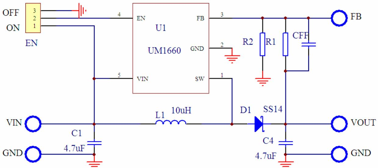
Fig 1.1 UM1660 EVB board schematic
