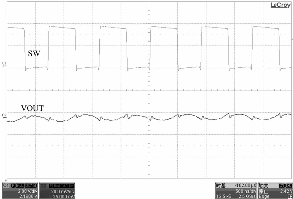
Fig 2.1 UM3501 waveform diagram ( $V_{IN}=3.6V$ ,  $V_{OUT}=1.8V$ ,  $I_{LOAD}=300mA$ )
