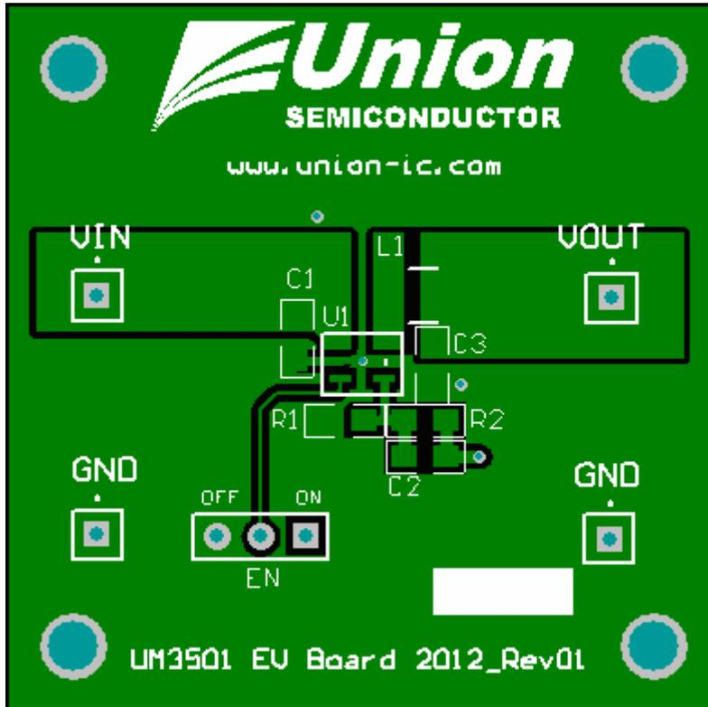
Fig 1.2 UM3501 EV board PCB top layer
