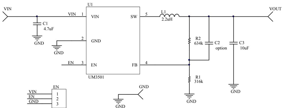
Fig 1.1 UM3501 EVB schematic
