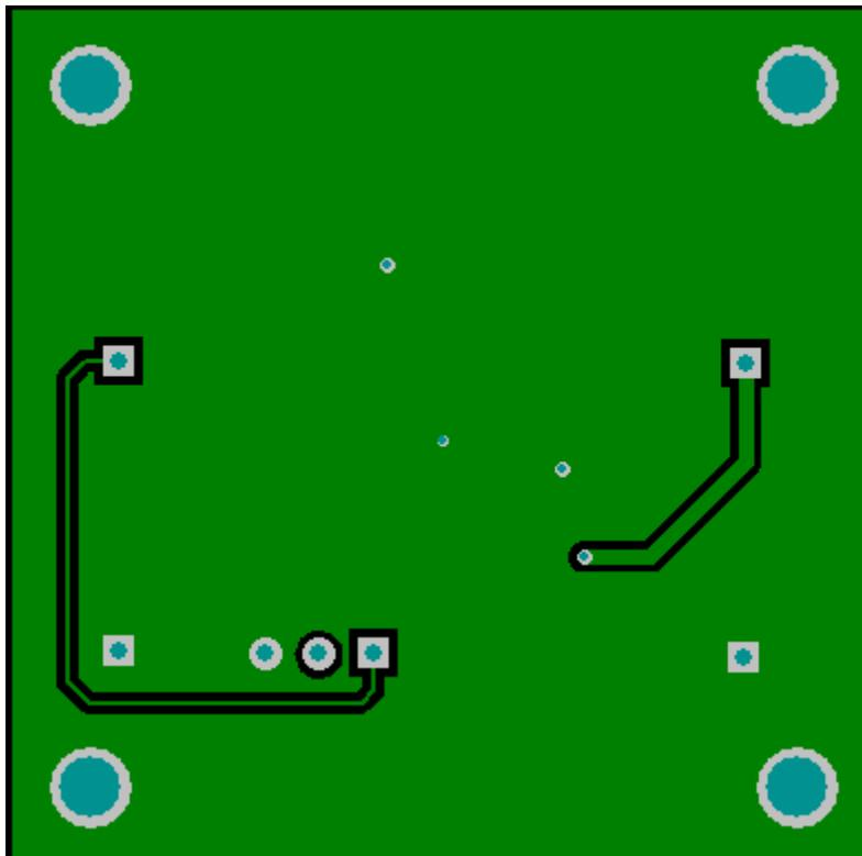
Fig 1.3 UM3501 EV board PCB bottom layer
