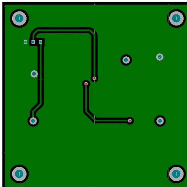
Fig 1.3 UM1661 EVB board PCB bottom layer
