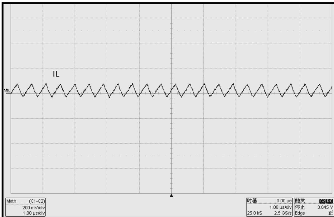
Fig 2.2 Inductor current waveform diagram
