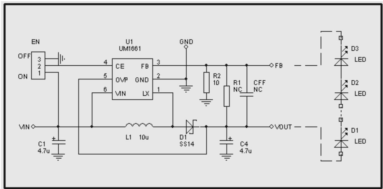
Fig 1.1 UM1661 EVB board schematic
