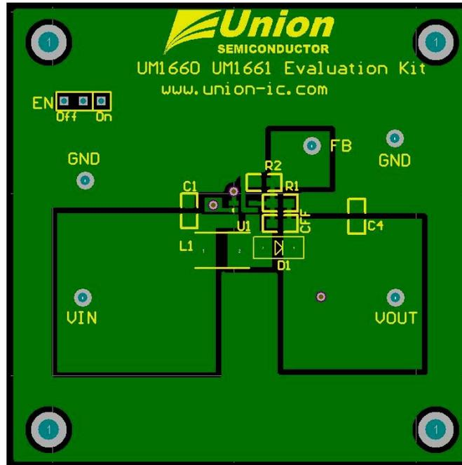
Fig 1.2 UM1661 EVB board PCB top layer
