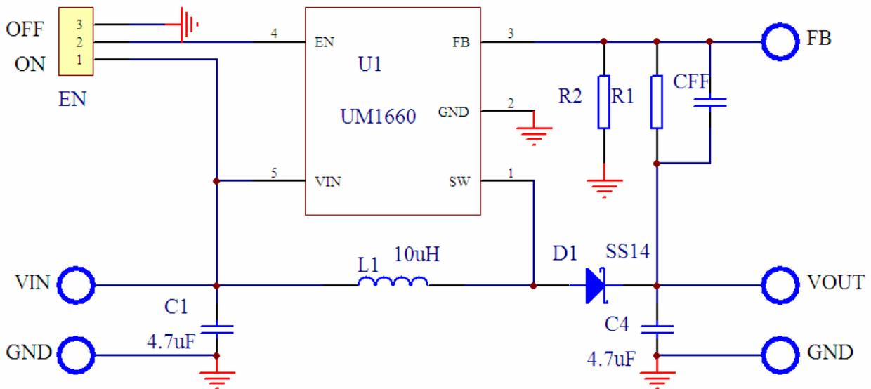
Fig 1.1 UM1660 EVB board schematic
