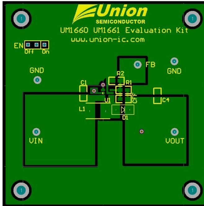
Fig 1.2 UM1660 EVB board PCB top layer
