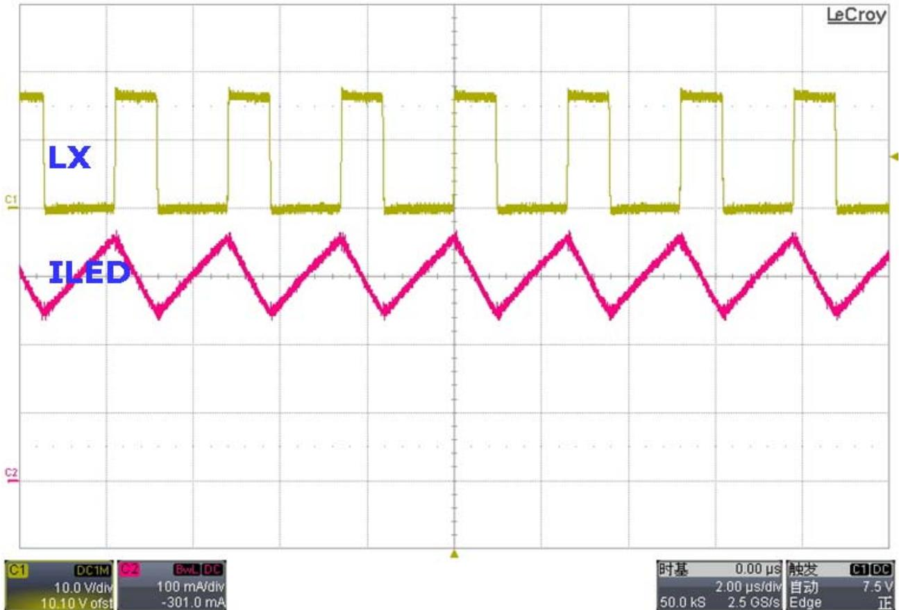
Fig 2.1 Typical Switching Operation Waveforms (3 LEDs,100uH,Vin=16V,Rs=0.33 Ω)
