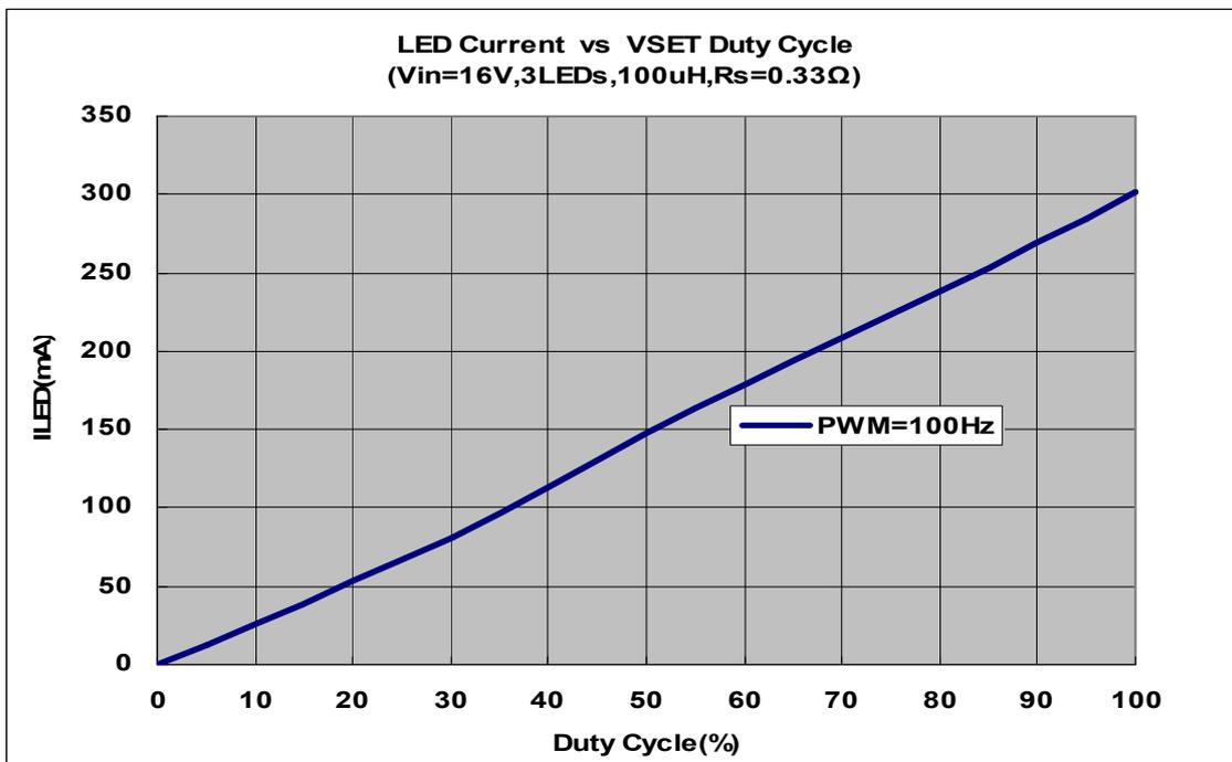
Fig 2.3 PWM Dimming
