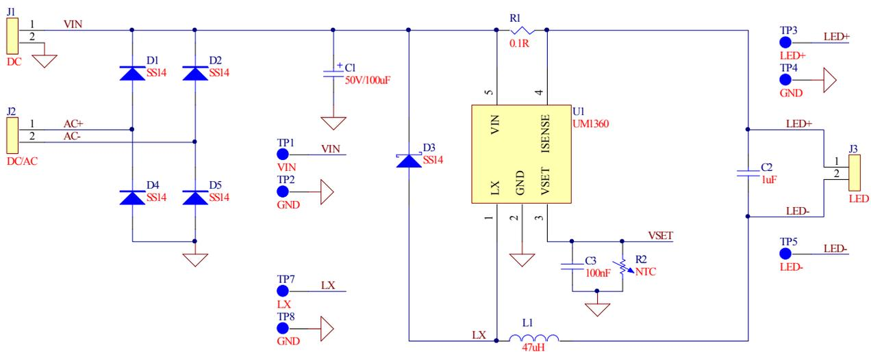
Fig 1.1 UM1360 EVB schematic
