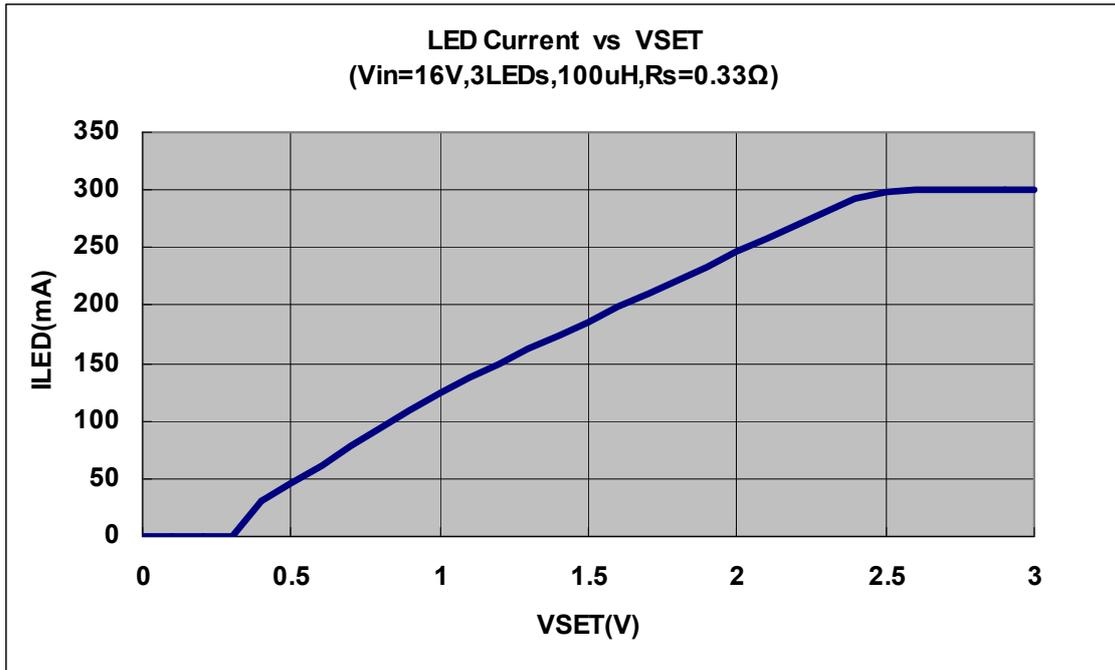
Fig 2.2 DC Dimming
